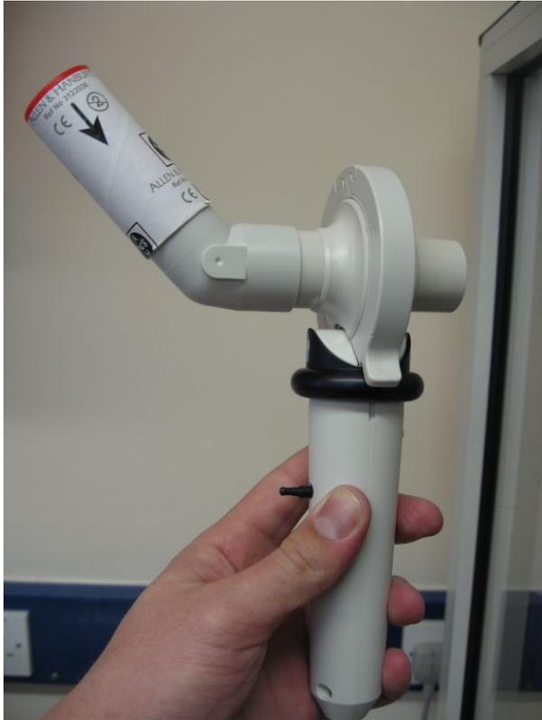
**Figure 2.3 Jaeger Masterscope® spirometer fitted with elbow piece and disposable mouthpiece**
